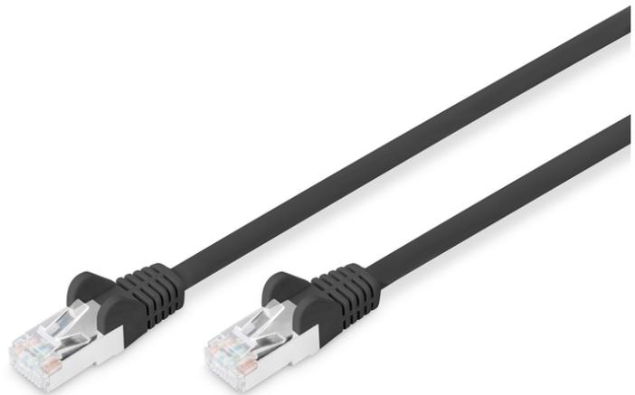
**Patchkabel, CAT6, RJ45 St/St, 5.0m, S-FTP, AWG 27/7, LSZH, sw**
