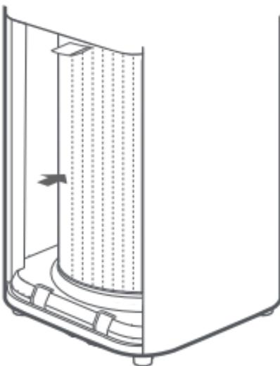
Install the filter into position with the filter strap on the top, then close the filter compartment.
