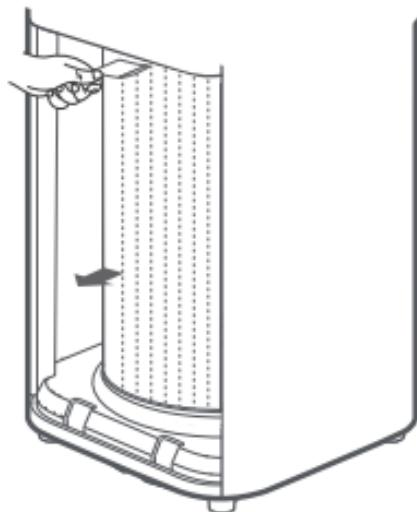
Pull the filter strap to remove the filter.
