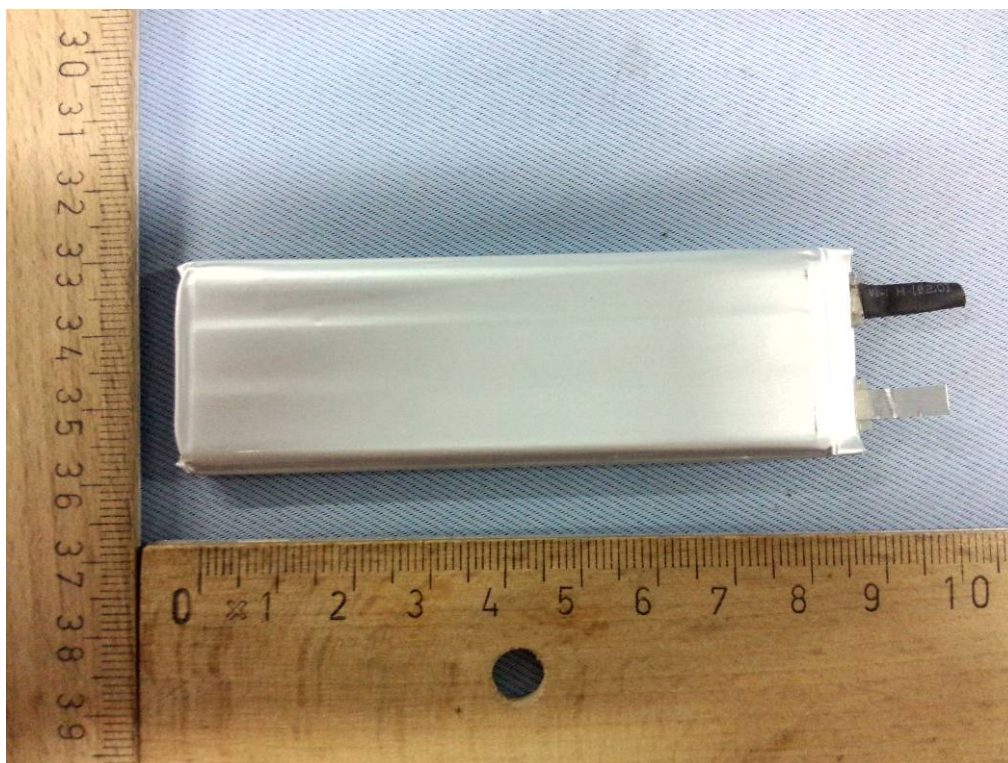
Inner Cell/内部电芯 ( 3,7V 1200mAh )
