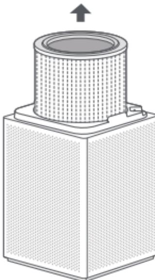
Remove the old filter upwards.
