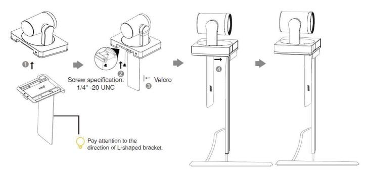
Choose the following installation method when the thickness of the TV is between 46 mm and 146 mm.
